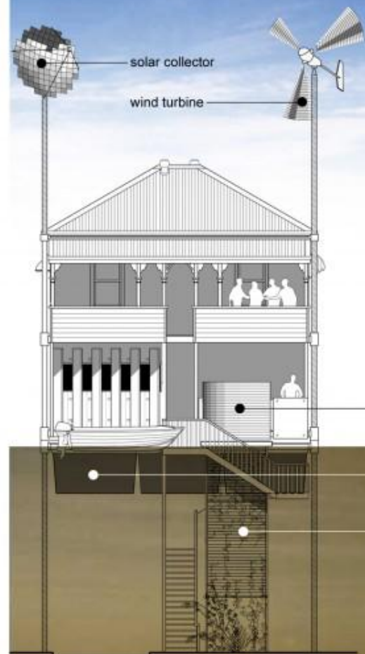
future flood level pontoon deck lifts house above the flood
