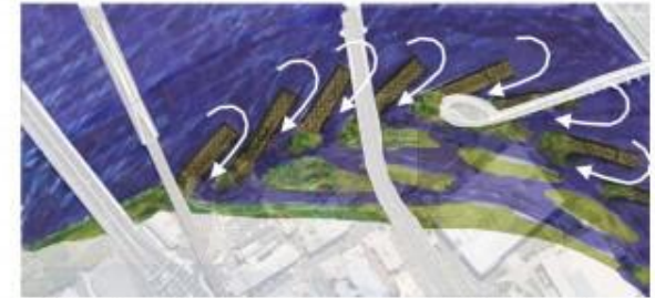
Tidal surge inundates terrain and scours non-vegetated areas, creating an-branching and forming islands.
