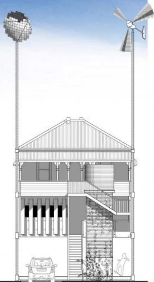
before the flood pontoon deck sits at ground level
