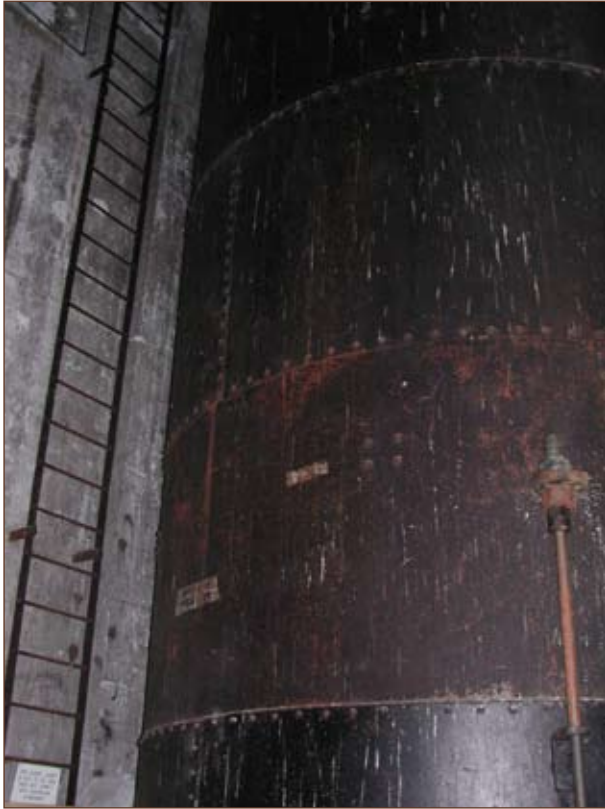
The accumulator - "I used to get up there and get in that big pot, and go up and down with the pot as it went up and down with the pressure "
