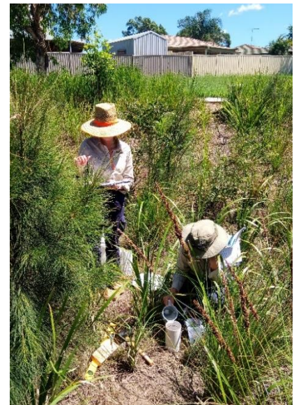
Testing infiltration rates at Fail Park Bioretention System
