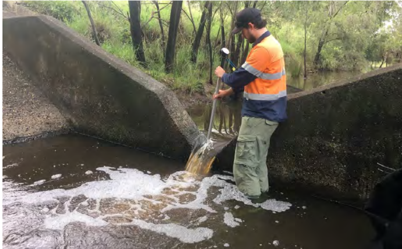
Figure 4. Measuring the velocity through the concrete v-notch gauging station barrier at Walloon in the lower reaches of the Bremer River.
