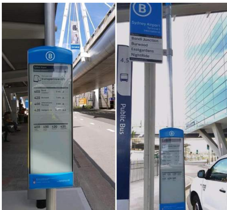
FIGURE 20: A dynamic real time passenger information screen at a bus stop at Sydney airport.
