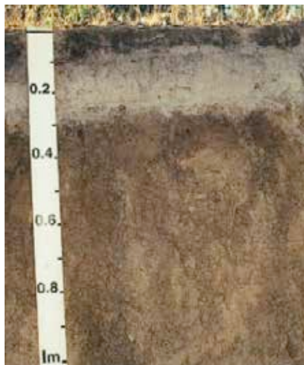
Sandy pale subsurface from 0.1m to 0.3m Source: Queensland Government (DSITIA)
