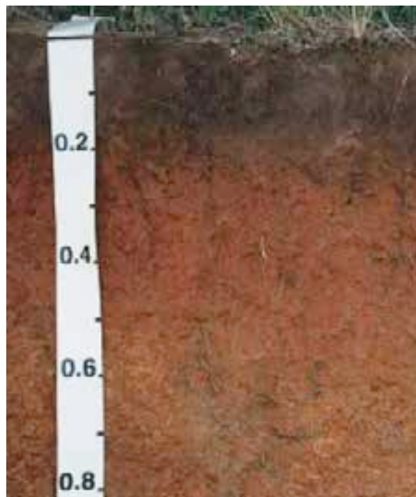
Red Chromosol with well structured subsoil Source: Queensland Government (DSITIA)
