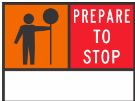
Figure 4.2.2 – Traffic Controller Ahead / PREPARE TO STOP Sign
