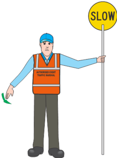
Figure 4.3.4(b) – Signal to SLOW traffic
