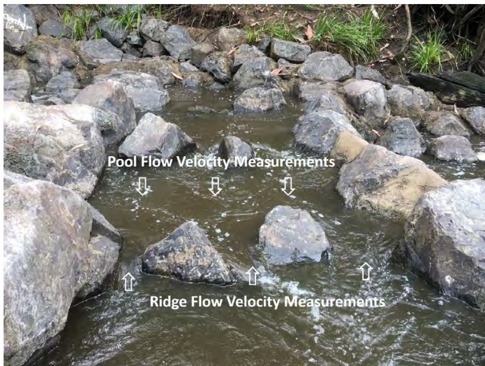
Figure 2. Image displaying locations of flow velocity replicates when taking fishway flow velocity readings, with one replicate in each of the three ridge slots and three replicates in each pool
