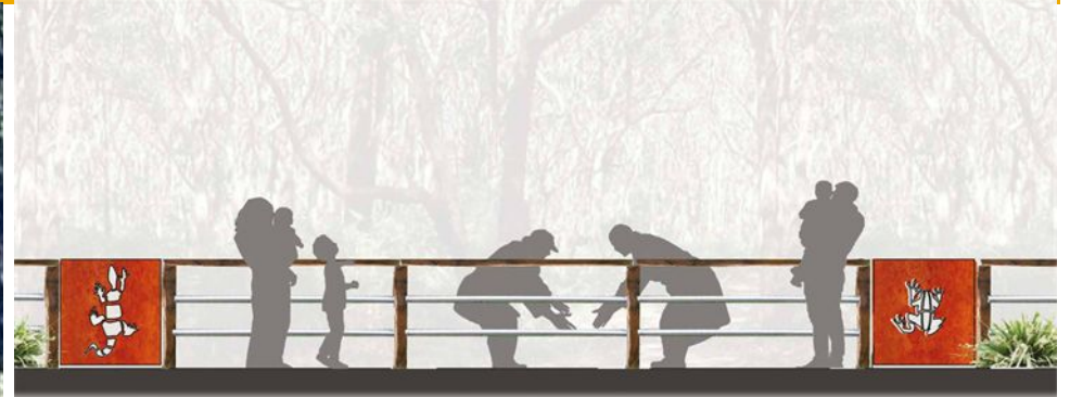
FENCE: 1200H Timber posts with twin gal pipe rails and plank top & laser cut panels
