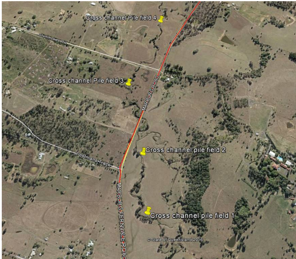
Figure 3 cross channel pile fields and locations to in channel water velocities and encourage sediment deposition to raise the creek bed level
