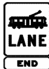
End tram lane sign
