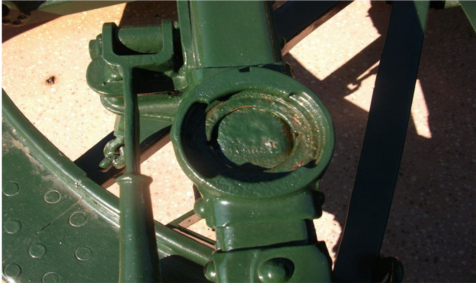
Chassis Left Rear – Area of chassis with rust developing through the paint. Requires rust removal, re-priming and repainting.
