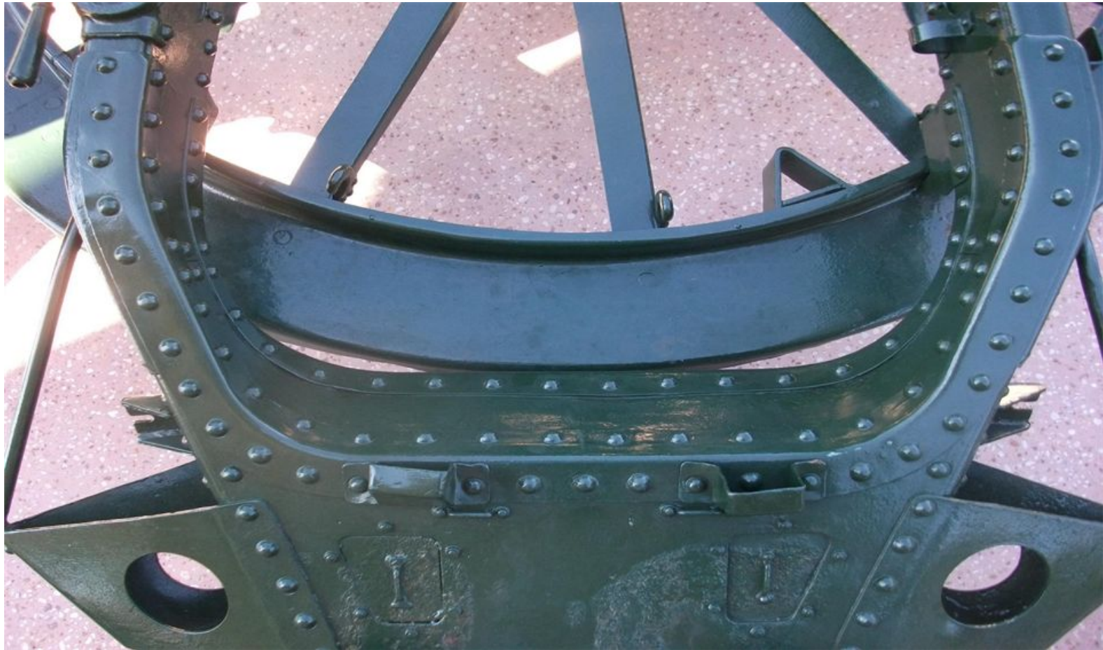
Rear Chassis lower seam (near Traverse Mechanism) – Requires to be sealed to prevent further chance of rusting.
