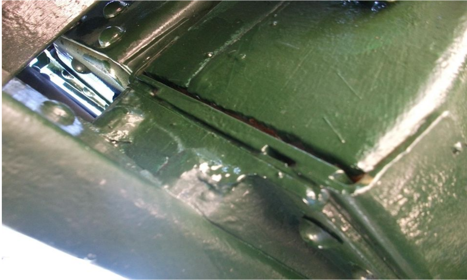
Underside of forward chassis – The left and right hand sides appear not to have been painted and are developing rust. Requires rust removal, re-priming and repainting.
