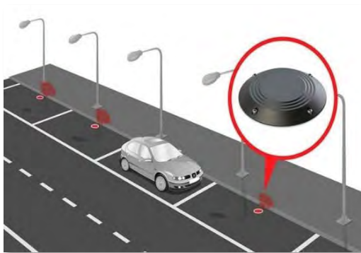
FIGURE 19: On-street Parking Sensors
