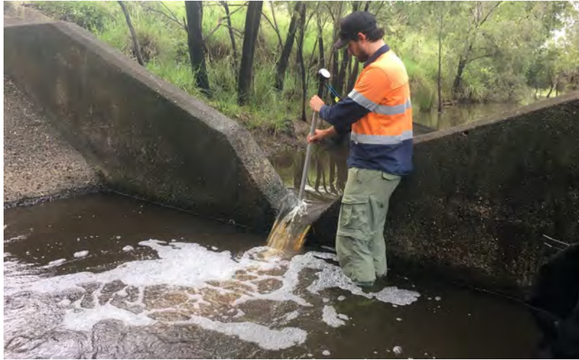
Figure 4. Measuring the velocity through the concrete v-notch gauging station barrier at Walloon in the lower reaches of the Bremer River.
