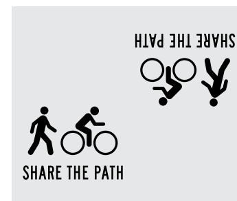
PBM-A Path behaviour pavement markings Example shows a 2.5m shared path without a centreline
