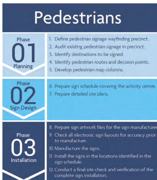
Figure 19: Planning a directional signage system for pedestrian activity centres
