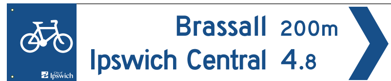
FBP-2 Two-line fingerboard layout for distances less than a kilometre.
