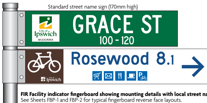
FDR Destination indicator fingerboard with additional wayfinding information on lower line - artwork template
