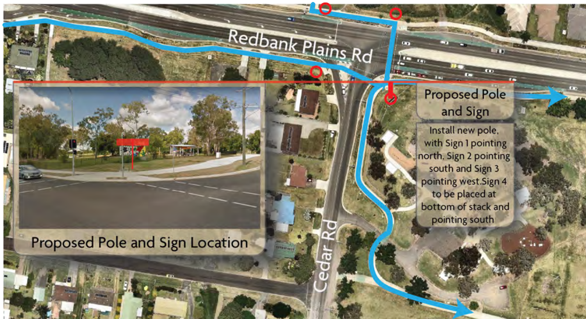
Figure 18: Example of a detailed Site Implementation Plan (Redbank Plains)
