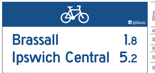
RDP-2 Two-line reassurance direction sign - artwork template
