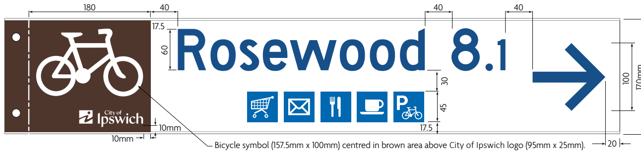
FIR Facility indicator fingerboard with pictograms (max 6) on lower line - artwork template See Sheets FBL-1 and FBR for typical fingerboard reverse face layout.
