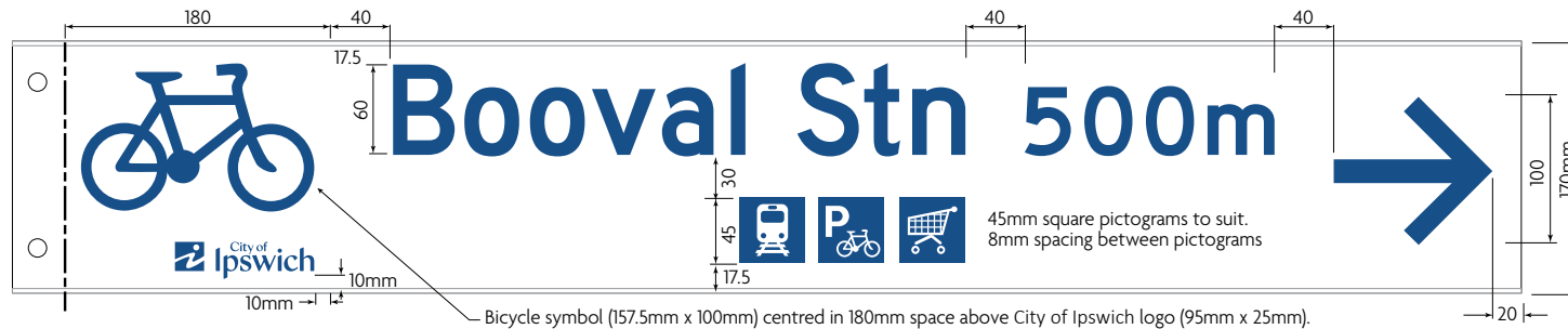
FBL-F Facility indicator fingerboard with pictograms (max 6) on lower line - artwork template See Sheets FBP-1 and FBP-2 for typical fingerboard reverse face layouts.
