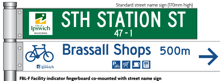
FBL-F Facility indicator fingerboard co-mounted with street name sign
