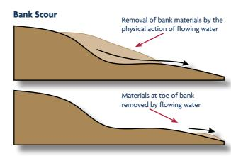
**Scouring** - often occurs at the toe of a bank (i.e. at the water's edge) where flowing water scours or washes away the bank soil. Scouring is also common on the outside bend of a waterway where the flow is at its fastest. Native vegetation along the waterway protects the bank against scouring by slowing the speed of water and providing a buffer (protective layer) over the soil. Scouring often removes soil around tree roots causing the tree to fall and remove a large section of the bank soil.
