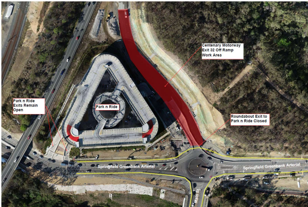
Diagram 1 – Work Area Centenary Motorway Exit 32 Off Ramp
