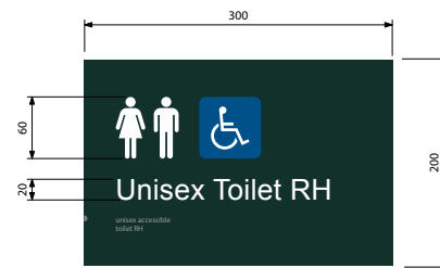
UNISEX ACCESSIBLE TOILET Braille translation = unisex accessible toilet RH (handing to be confirmed)
