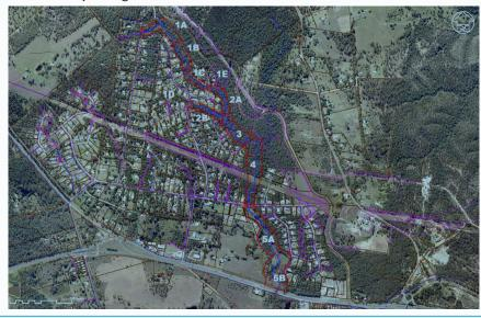
All sections of Ironpot Creek studied are experiencing some degree of erosion. This may be in the form of bank scour, bed lowering and or head cuts with the most significant erosion sites located within Management Zones 1b, 2a and 3 (see above study area map for zone locations). While some of these erosion sites will stabilise naturally, there are instances where channel adjustments (e.g. stream widening) are not acceptable and therefore coordinated management intervention may be required.
